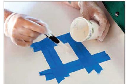
Use a mixing stick to run the gelcoat into the crack.
